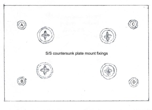
A,B,C & D vertical S/S all-thread balustrade mounting spigots 'tig' welded onto 5mm S/S base plate (to be recessed into substrate)
